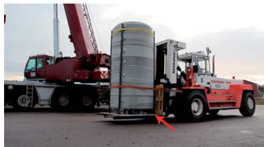
FIG. 3. A fully assembled distance block, the cable block can be seen at the bottom of the component (marked with a red arrow).
