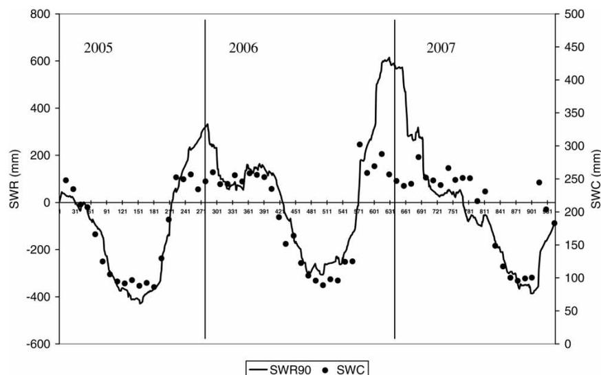
**Figure 3** | Soil water reserve (SWR) estimated (line) and soil water content (SWC) measured (dots) from April 1 (DOY 1), 2005 until October 31, 2007.
