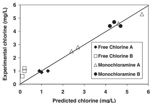
**Figure 7** Predicted and experimental chlorine concentrations at end of pass 1
