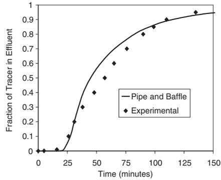
**Figure 4** Predicted tracer curve for pass 1 of reactor
