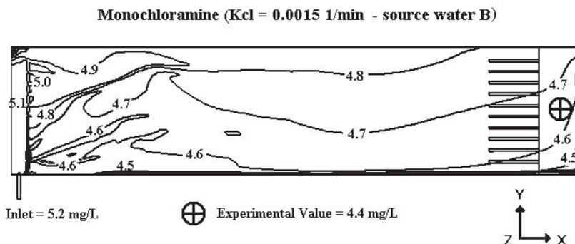
**Figure 6** Predicted monochloramine concentration contour plot
