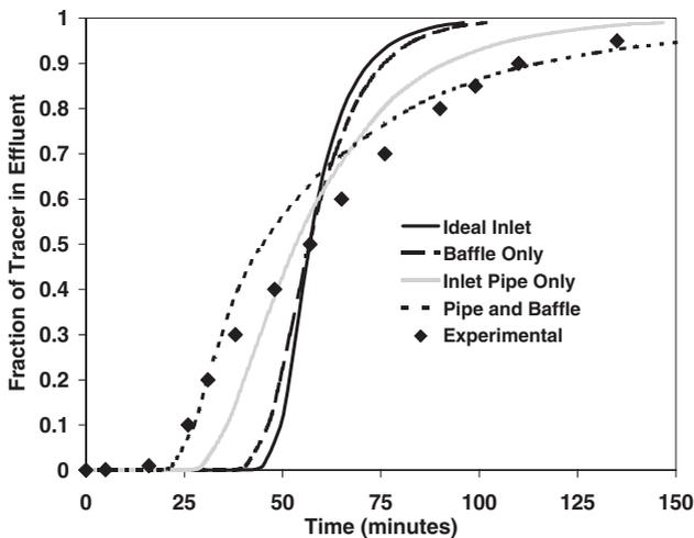
**Figure 5** Predicted tracer curves for alternative inlet configurations
