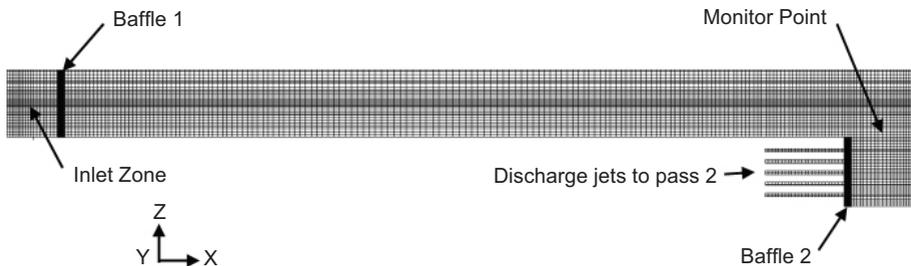
**Figure 2** Computational model – Pass 1 (reactor plan view)
