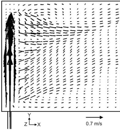
**Figure 3** Predicted flow structure for reactor inlet region
