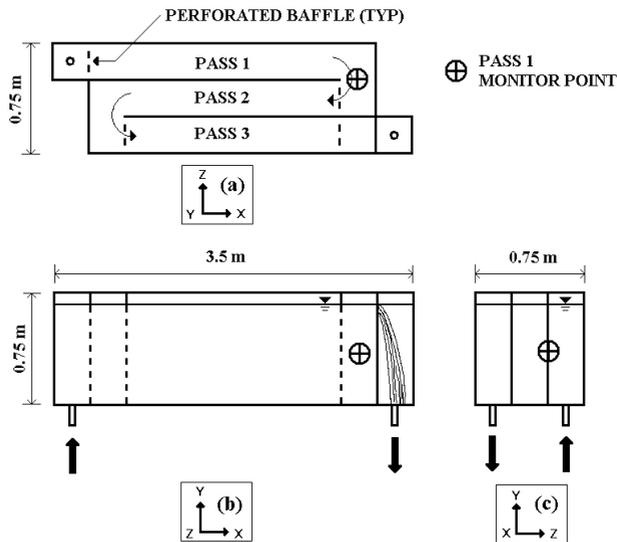
**Figure 1** Pilot scale reactor configuration: (a) plan view; (b) profile view; (c) side view
