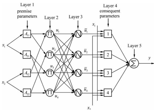
Figure 2 | Two-input ANFIS with four rules.
