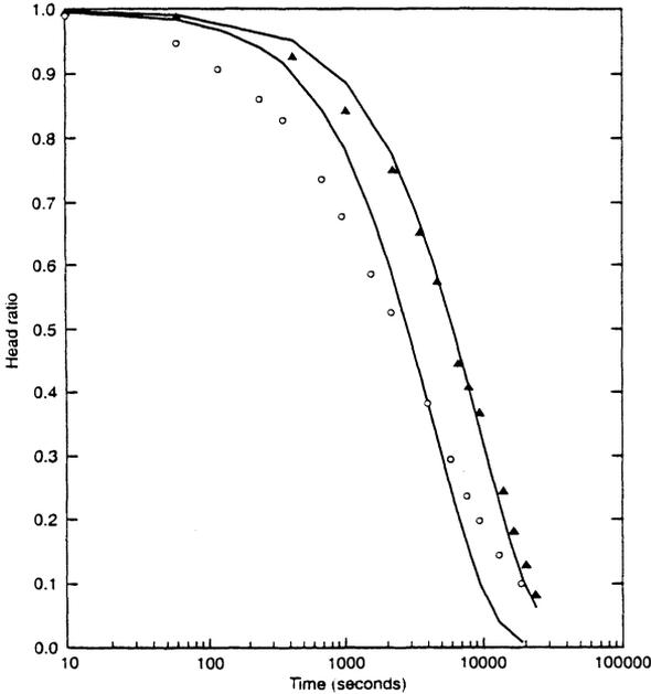
Fig. 2. Example head recoveries. Closed triangles are for piezometer  $A_{120}$  on site 1, open circles for piezometer  $C_{200}$  on site 2. The solid lines are fitted responses (least differences) according to Eq. (1).
