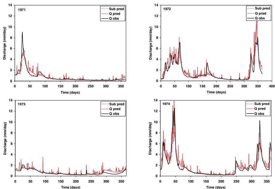
**Figure 2** Examples of predicted ( $Q_{pred}$ ) versus observed ( $Q_{obs}$ ) daily runoff for the Slapton Wood catchment for 1971, 1972, 1973 and 1974.  $Sub_{pred}$  is the predicted sub-surface flow component
