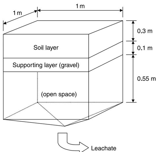
Figure 4 | Schematic diagram of a lysimeter.
