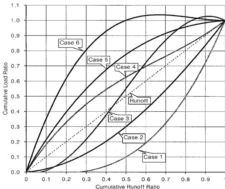
**Figure 6** Shape of first flush curves with polynomial equation constants
