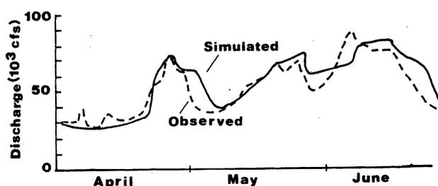
Fig. 5. Comparison of modified model results between observed and simulated yields for the Kabul basin  $5^{\circ}\text{F}/1,000 \text{ ft}$  ( $0.98^{\circ}\text{C}/100 \text{ m}$ ) normal lapse rate and 8,500 ft (2,591 m) mean elevation of the watershed.
