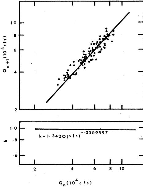
Fig. 3. Regression flow plot  $Q_n$  versus  $Q_{n+1}$ , and relation of  $k$  and  $Q$  for the Kabul Basin.
