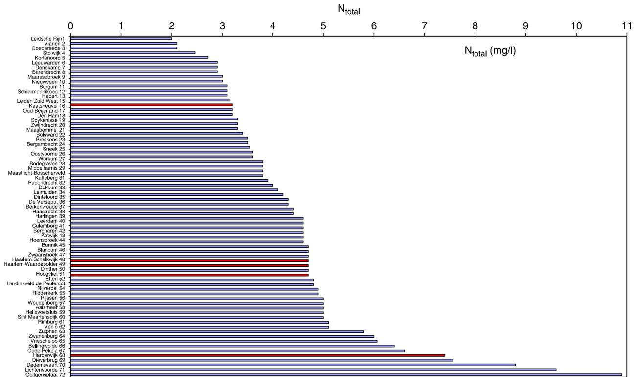
**Figure 2** Yearly average  $N_{total}$ -concentration in effluent of identified WWTP's (year 2005). Subscribers to the online version of *Water Science and Technology* can access the colour version of this figure from <http://www.iwaponline.com/wst>
