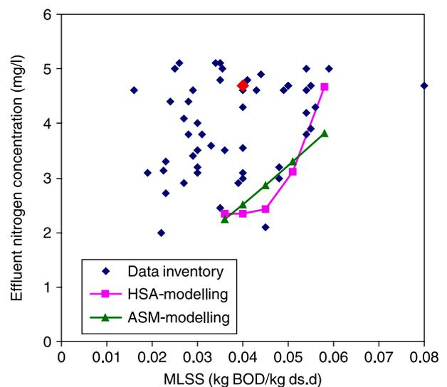
Figure 4 | Comparison of practical results ( $\diamond$  = WWTP Hoogvliet) and model based results—MLSS-concentration. Subscribers to the online version of *Water Science and Technology* can access the colour version of this figure from <http://www.iwaponline.com/wst>
