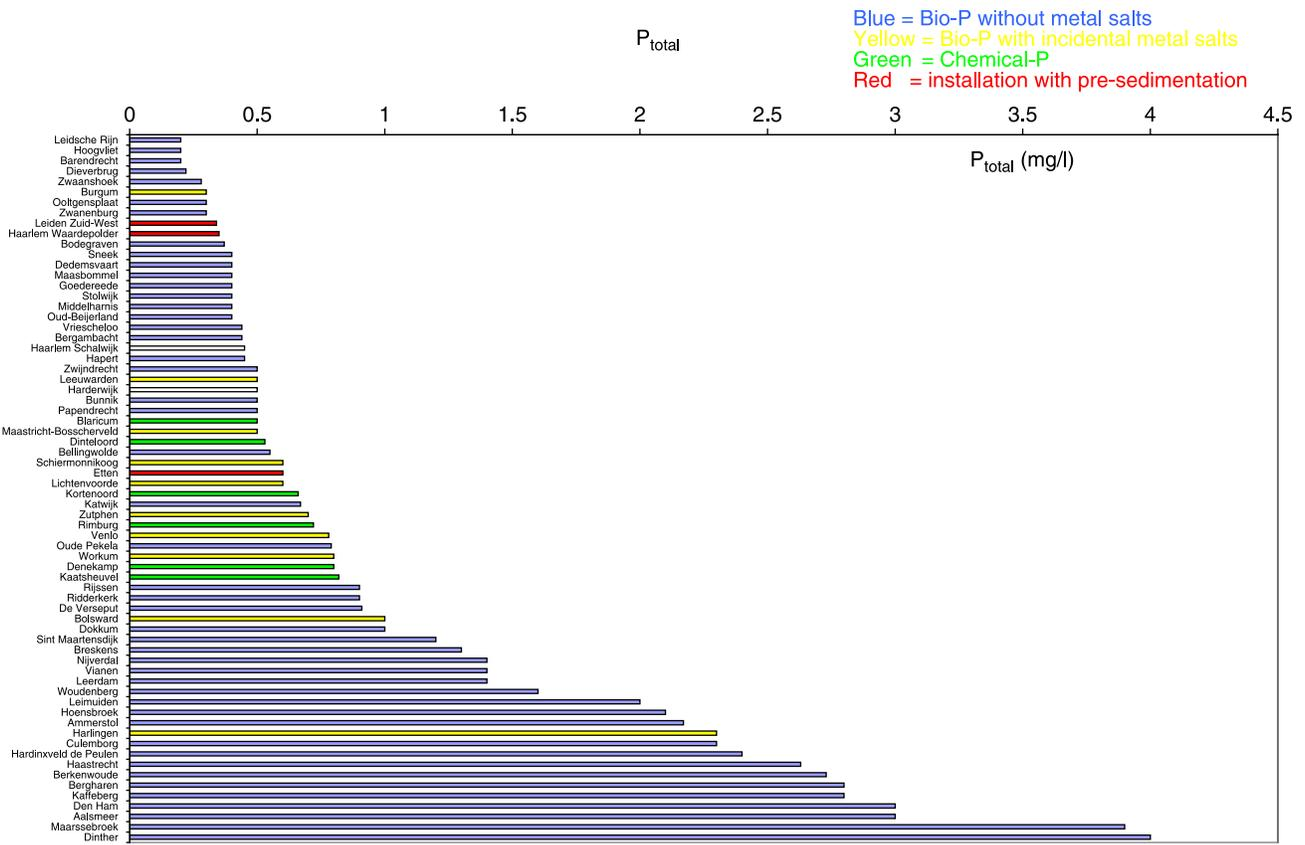
Figure 3 | Yearly average  $P_{total}$  concentration in effluent of identified WWTPs (year 2005). Subscribers to the online version of *Water Science and Technology* can access the colour version of this figure from <http://www.iwaponline.com/wst>
