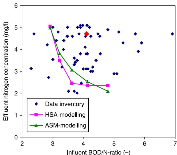
**Figure 5** | Comparison of practical results and ( $\diamond$  = WWTP Hoogvliet) and model based results—BOD/N-ratio. Subscribers to the online version of *Water Science and Technology* can access the colour version of this figure from <http://www.iwaponline.com/wst>
