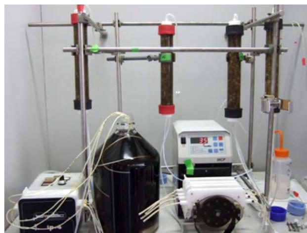
**Figure 1** | Picture of the Pyrex glass reactor filled with polyethylene rings employed for Biodegradation experiments.
