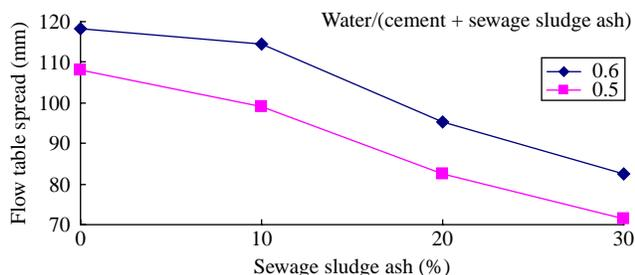
Figure 1 | Variation of flow table spread values versus sewage sludge ash percentage.
