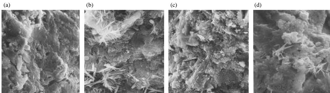
**Figure 3** | SEM images of sludge ash mortar at 28 days curing age. (a) Control mortar; (b) 10% sludge ash mortar; (c) 20% sludge ash mortar and (d) 30% sludge ash mortar.
