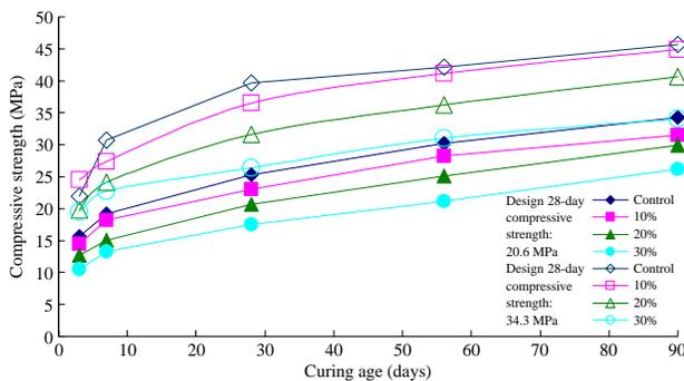
Figure 4 | Compressive strength of sewage sludge ash concrete.
