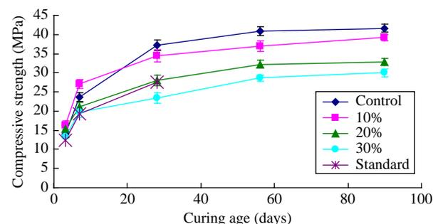
Figure 2 | Compressive strength of hardened sewage sludge ash mortar.
