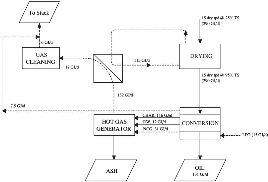
**Figure 2** Energy balance for integrated demonstration plant
