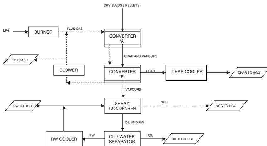
**Figure 1** Conversion plant process flow diagram
