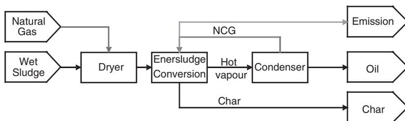
**Figure 4** Simple flowsheet for nutrient and energy recovery
