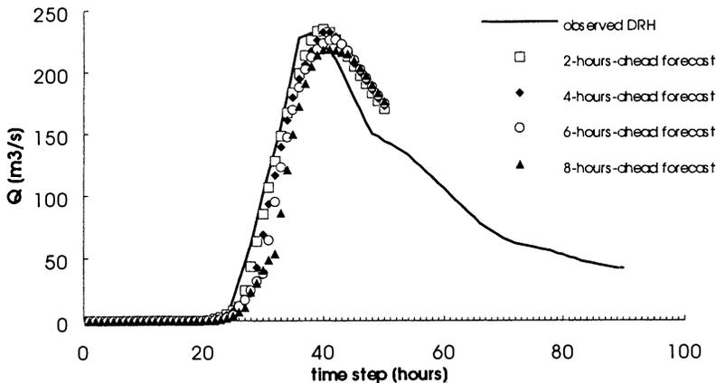
Fig. 6. Observed direct runoff hydrograph and 2-4-6-8 hours ahead forecasts by means of the on-line optimization of the initial condition  $C^*_0$  for the May 1977 event (the value of  $\sigma$  was assumed to be 270 mm).
