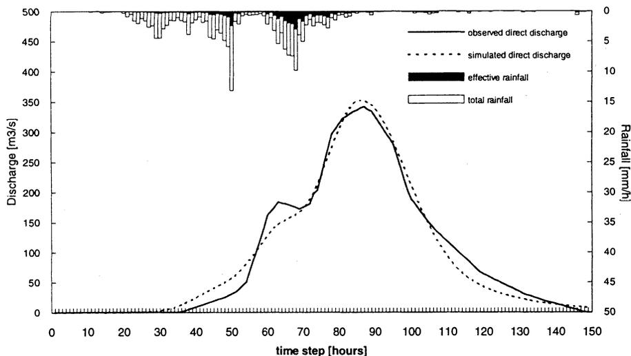
Fig. 2. Observed and simulated direct discharge after the off-line automatic calibration for the November 1941 event (estimated values:  $\sigma = 362$  mm,  $C^*_0 = 83$  mm).
