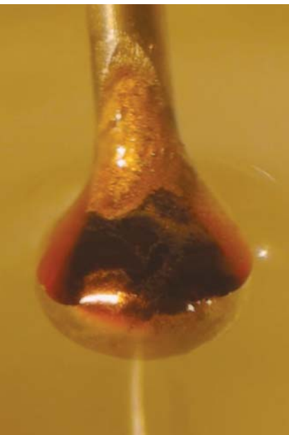
FIGURE 1. ALKALI METAL–AMMONIA SOLUTIONS are a deep blue color at concentrations below about 4 mol percent metal. At higher concentrations their electrons transition from localized to extended states, which causes the solutions to turn bronze and exhibit metallic behavior. (Courtesy of Philip Mason.)
