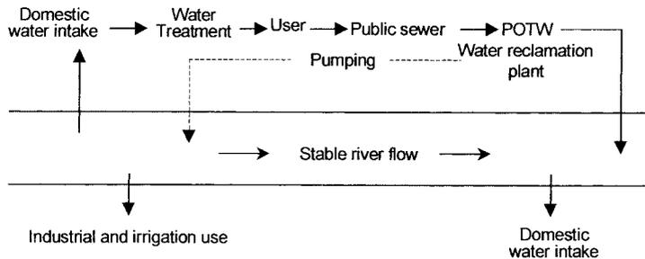
**Figure 2** Water recycling system schemes used in Japan
