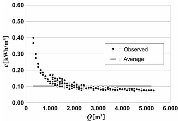
Figure 1 | An example of electric power consumption rate [kWh/m<sup>3</sup>].
