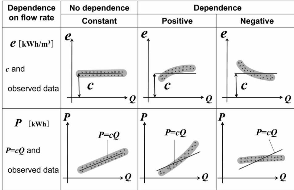
Figure 3 | Relation of energy consumption rate and electric power usage to flow rate  $Q$ .
