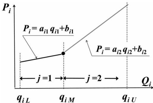
Figure 4 | Equation used to estimate electric power usage at facility  $i$  for water flow rate range  $j$ .
