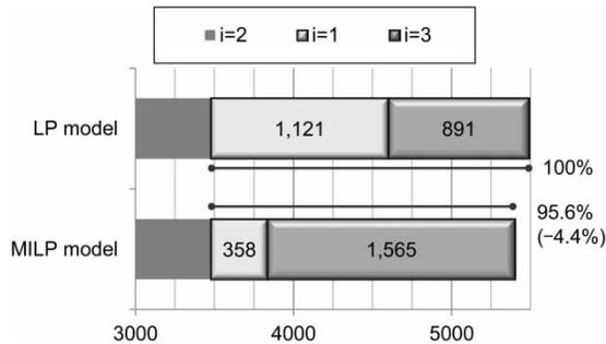
**Figure 10** | Comparison of electric power usage [kWh/h] with the MILP model and LP model (at time  $t = 1$ ). The values for electric power usage in the case of the LP model are based on the same estimation equation as that used in the MILP model for calculating power usage. It should be noted that the results for electric power usage by facility  $i = 2$  are the same with both models.
