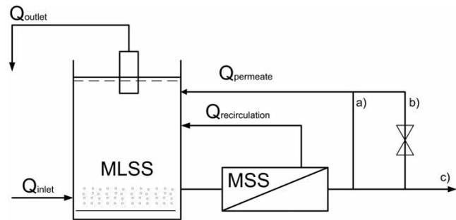
**Figure 1** | Overview of test setup to expose activated sludge to shear from GBB membranes (test a) and the pressure reduction component (test b). MSS: membrane suspended solids.
