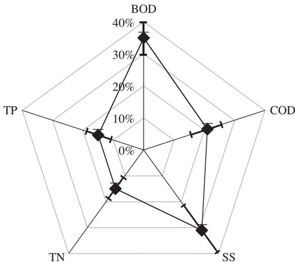
**Figure 4** Net overall reduction of the total pollutant discharge during storm events by passing to high-flow AS operation at STP Ertvelde
