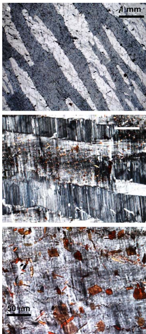
FIG. 1. Light micrographs of Hunterian M2361, probably the type perthite from Perth, Ontario. Crossed polarizers, section parallel to (001). (a) Low magnification image showing lenses of albite (white), with a conspicuous {110} cleavage, in microcline (grey). The microcline is crowded with black dots, which are biotite crystals. (b) Albite twinned albite lamellae slightly oblique to b and fine-scale 'tartan', combined Albite and Pericline twinning, in microcline. In places there is a clear interaction between Albite twins in both phases at the margins of the lamellae. Biotite flakes tend to be concentrated around the centre of the microcline lamellae, although they sometimes occur near margins and rarely in the albite. (c) Thin euhedral flakes of biotite in microcline with very fine-scale, regular tartan twins. The biotite does not influence the twinning in any way.
