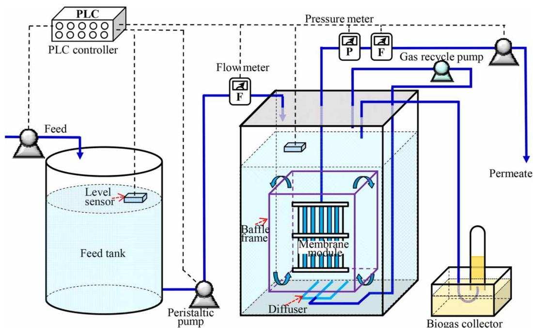
Figure 1 | Schematic diagram of the experimental AnSMBR setup.
