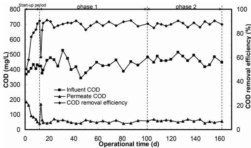
Figure 2 | Variations of influent COD, permeate COD and COD removal efficiency with operational time.
