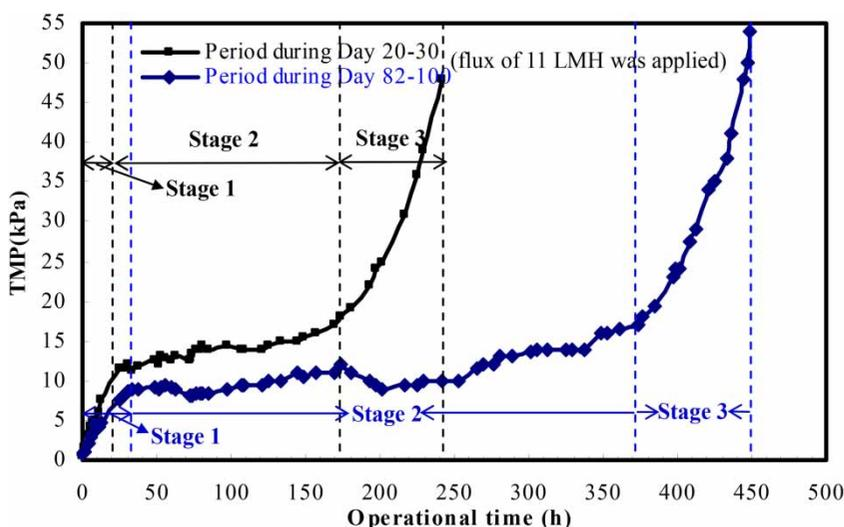
Figure 3 | Typical profile of TMP variation with operational time.
