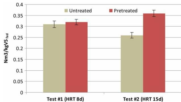
**Figure 2** | Specific biogas production (Nm<sup>3</sup>/kgVS<sub>fed</sub>) of untreated and thermal pre-treated sludge.
