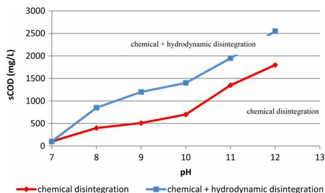
**Figure 1** | Release of soluble COD after chemical disintegration alone, and coupled with hydrodynamic cavitation.
