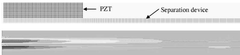
**Figure 7** Construction of acoustic pressure field in the separation channel (1/2 with symmetry)
