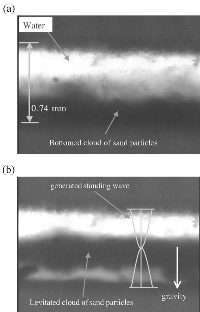
**Figure 10** Levitation of heavy sand particles cloud using ultrasonic standing wave: (a) before; (b) after
