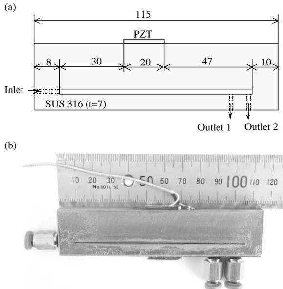
**Figure 4** The separation device: (a) design and dimension; (b) photograph
