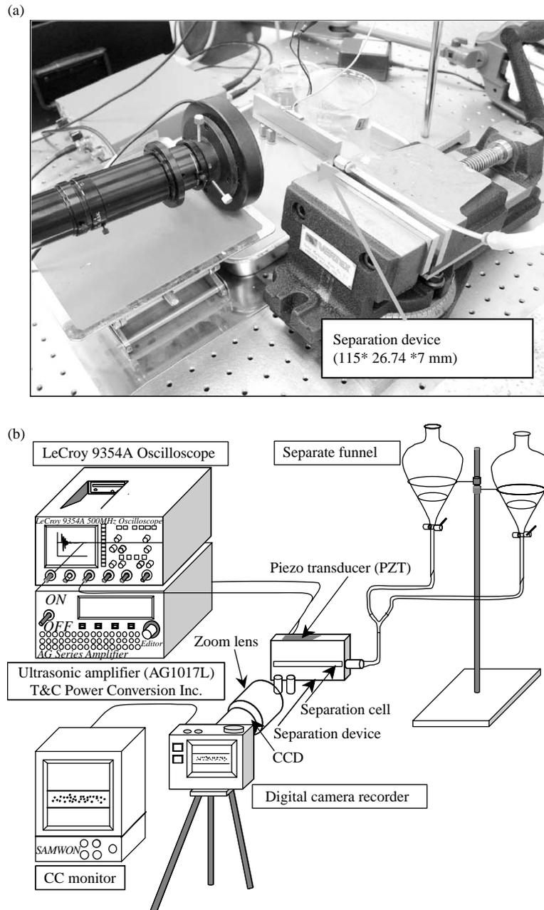
**Figure 9** Experimental set-up with the smart separation device: (a) photograph; (b) separation test arrangement
