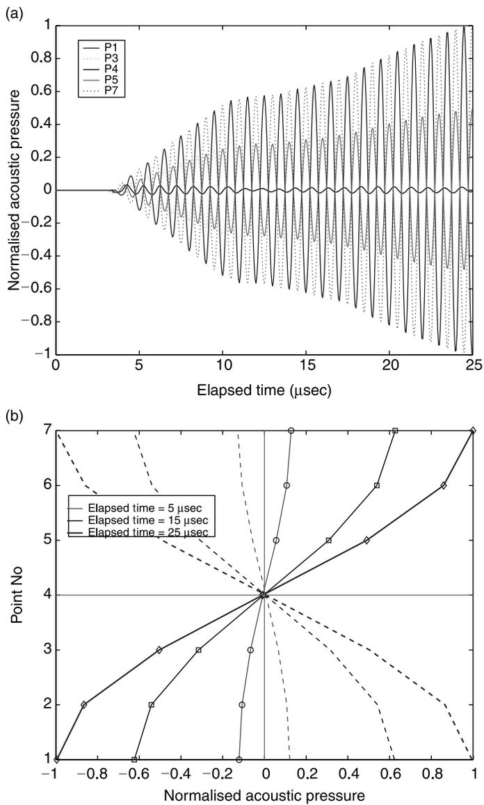
**Figure 6** Finite element analysis results: (a) pressure field vs elapsed time; (b) standing wave formation with time
