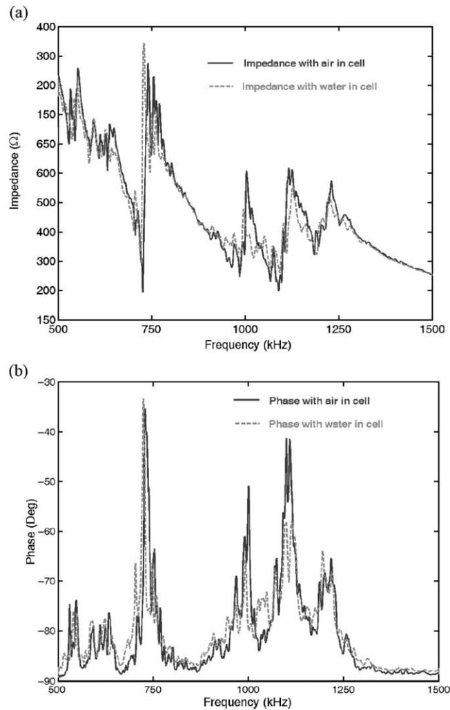
**Figure 8** Measured impedance of the PZT patch bonded on the smart separation device
