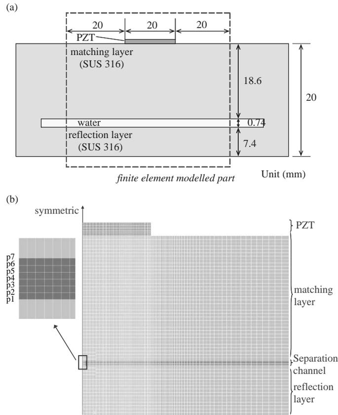
**Figure 5** Finite element model: (a) modelled part; (b) modelling (1/2 with symmetry)
