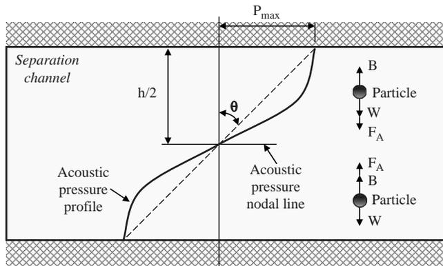
**Figure 2** Pressure gradient and exerting forces at particles in acoustic separation device
