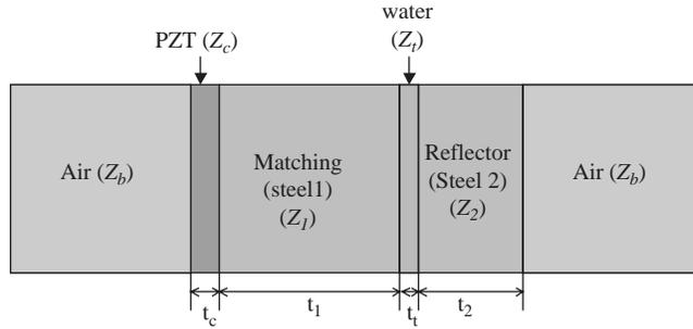
**Figure 3** Schematic diagram of ultrasonic separator for electro-acoustical analysis
