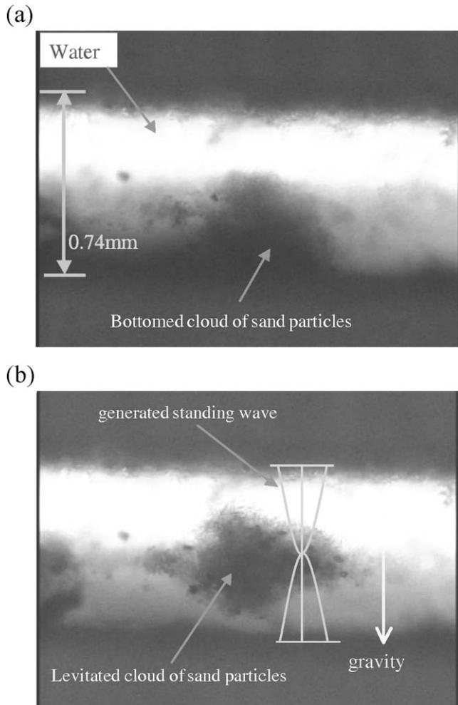
**Figure 11** Levitation of light sand particles cloud using ultrasonic standing wave: (a) before; (b) after
