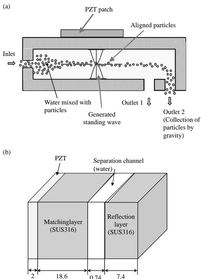
**Figure 1** A smart separation device with ultrasonic standing wave: (a) concept; (b) separator design
