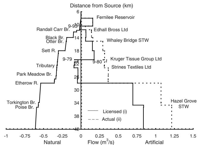
**Figure 7** | Annual residual flow diagrams of the Goyt river based on the  $Q_{95}(1)$  low flows of the Marple Bridge (no. 692015) flow station and (i) the licensed or (ii) the actual flows of the artificial sources in 1994.
