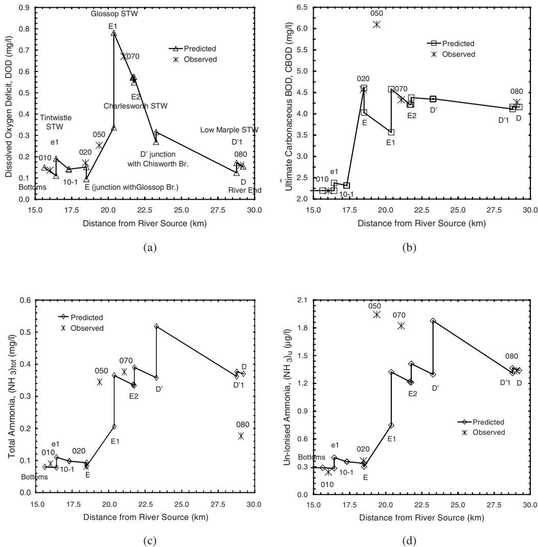
Figure 8 | Simulated and observed concentration of DOD, CBOD, (NH<sub>3</sub>)<sub>tot</sub> and (NH<sub>3</sub>)<sub>u</sub> along the Etherow River for the year 1994.
