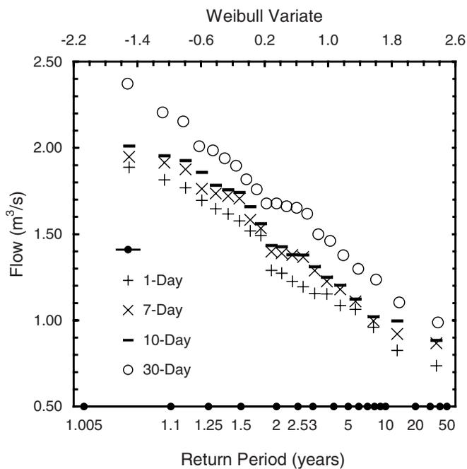
**Figure 5** | Low flow frequency curves drawn on Weibull probability paper of  $\varepsilon=0$  and  $k=4.0$  for the Portwood flow station (no. 692423) of the Tame River, for durations of 1, 7, 10, and 30 days.
