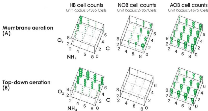
**Figure 3** AOB, NOB, and heterotroph cell counts as a function of bulk ammonia, oxygen, and carbon
