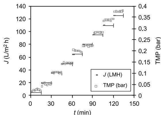
**Figure 3** Permeate flux ( $J$ ) and TMP range ( $u_{air} = 0.5$  m/s,  $TiO_2 = 10$  g/L)
