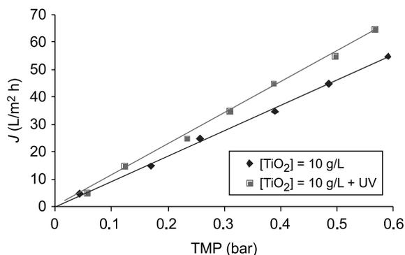
**Figure 7** Comparison of the microfiltration performance simultaneously with photocatalysis
