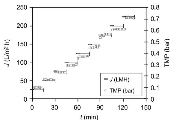
**Figure 2** Permeate flux ( $J$ ) and TMP range ( $u_{liq} = 0.5$  m/s,  $TiO_2 = 0$  g/L)
