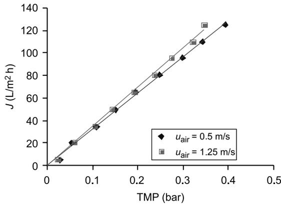
**Figure 4** Permeability graph for tests carried out with  $[TiO_2] = 5 \text{ g/L}$
