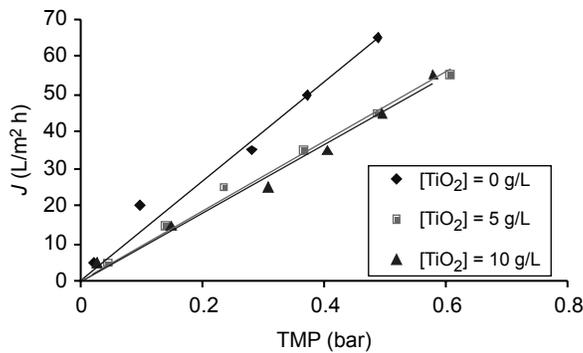
**Figure 6** Permeability graphs for grey water experiments carried out with different catalyst concentration ( $u_{air} = 0.5 \text{ m/s}$ )
