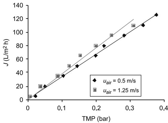
**Figure 5** Permeability graph for tests carried out with  $[TiO_2] = 10 \text{ g/L}$
