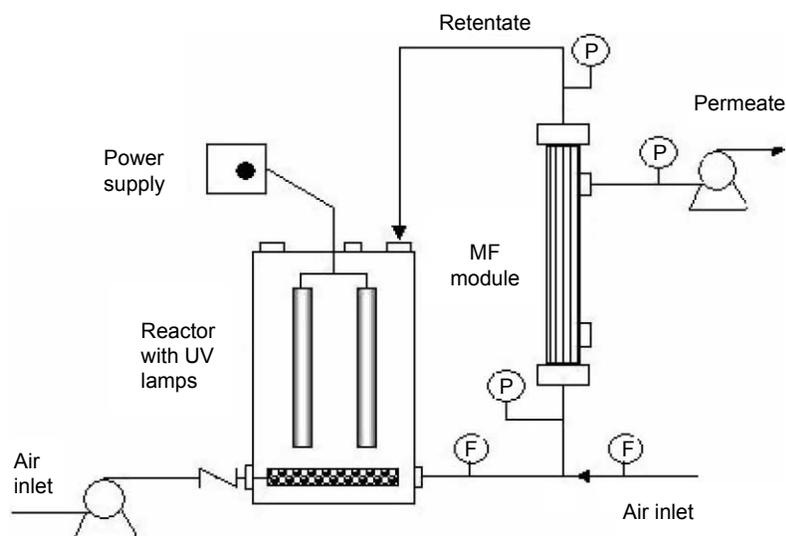
Figure 1 Diagram for the reactor system
