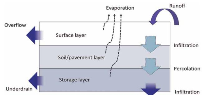
Figure 2 | Conceptual model of a LID process (Source: USEPA 2012).
