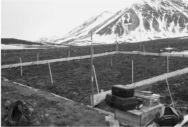
Figure 1 IH lower runoff plot after melt showing snow depth measurement positions, walls and drainage gutter, 25 June 1999
