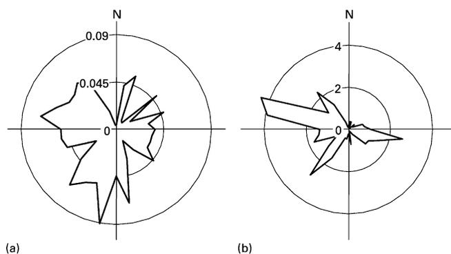
**Figure 8** Dependence of APM estimated latent heat flux on wind direction. (a) Average rate of evaporation ( $\text{mm h}^{-1}$ ), (b) total evaporation (mm). Roses are prepared using hourly data (895 points) and have plotting intervals of  $10^\circ$
