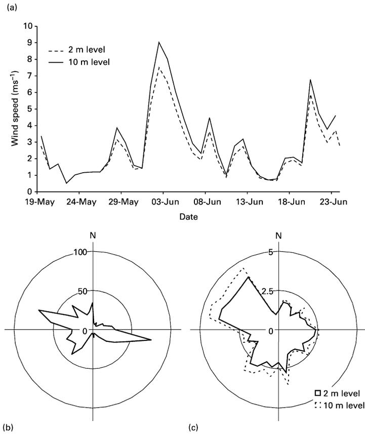
**Figure 2** Wind characteristics. (a) Average daily wind speed, (b) wind direction hourly frequency, (c) hourly wind speed ( $\text{m s}^{-1}$ ) as a function of wind direction. Roses are prepared using hourly data (895 points) and have plotting intervals of  $10^\circ$
