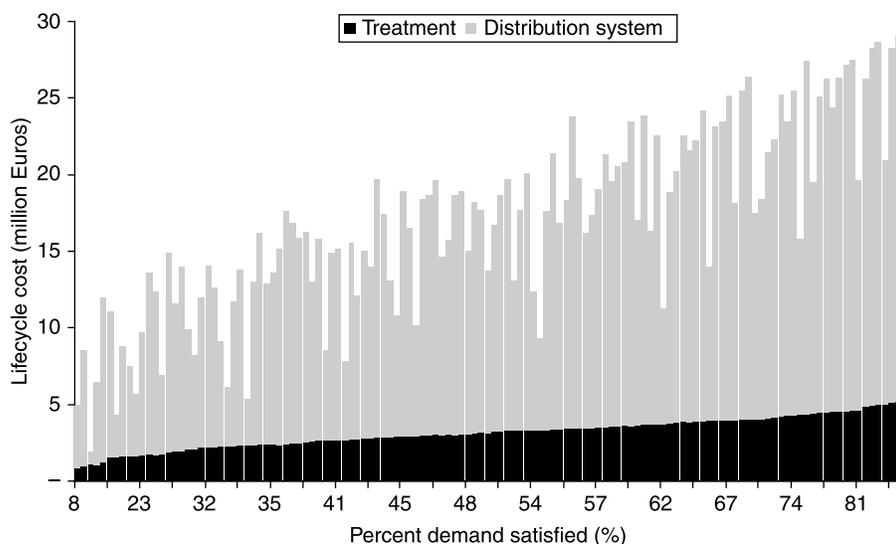
**Figure 4** Life cycle cost of different reuse scheme options
