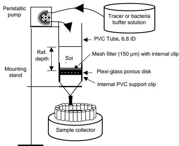
**Figure 1** Soil column setup
