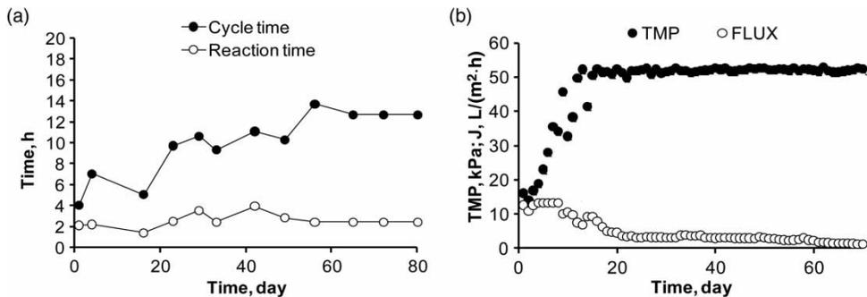
**Figure 4** | (a) Variation in cycle duration due to membrane fouling (note that reaction time was maintained constant) and (b) variation in transmembrane pressure (TMP) and flux during operation of the MSBR.
