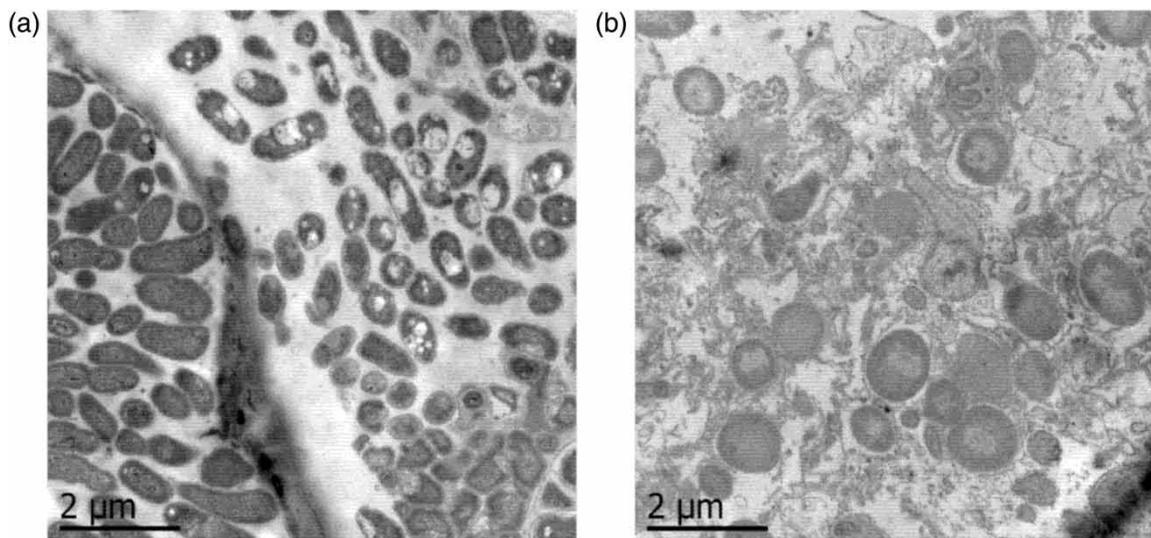
**Figure 7** | TEM images at day 15. (a) Superficial fouling biofilm on membrane; (b) transversal cut showing the cells inside the membrane (non-reversible clogging).
