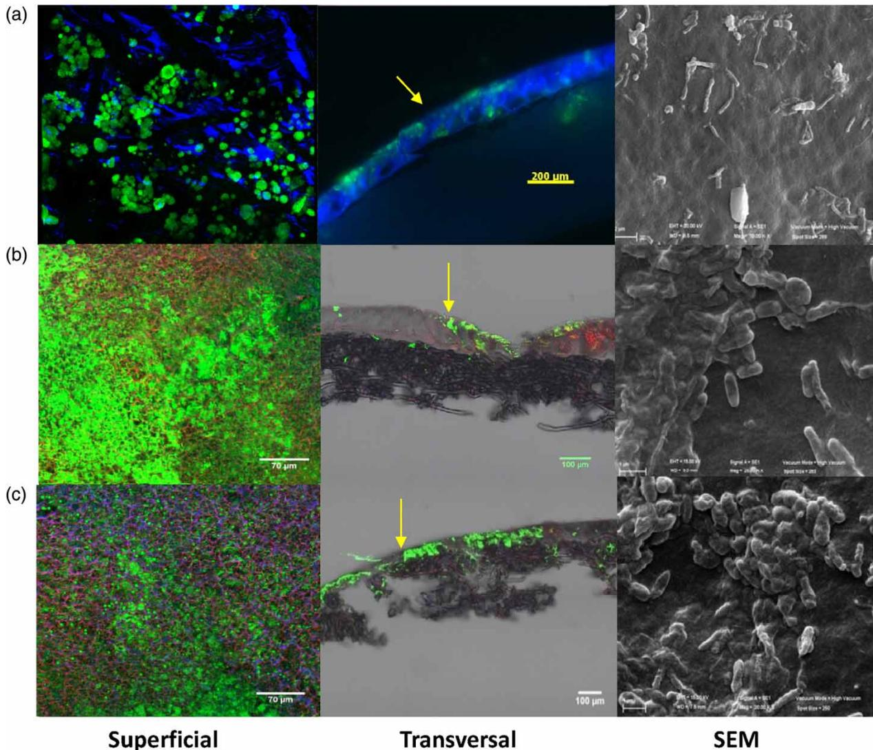
**Figure 5** | CLSM images of superficial and transversal sections of the membranes and superficial SEM images at (a) 10 d, (b) 40 d and (c) 60 d. For the superficial and transversal sections, white = proteins (green in online version), and blue = polysaccharides (blue in online version). Red = bacteria cells. Arrows indicate the membrane surface. The full color version of this figure is available online at <http://www.iwaponline.com/wst/toc.htm>.
