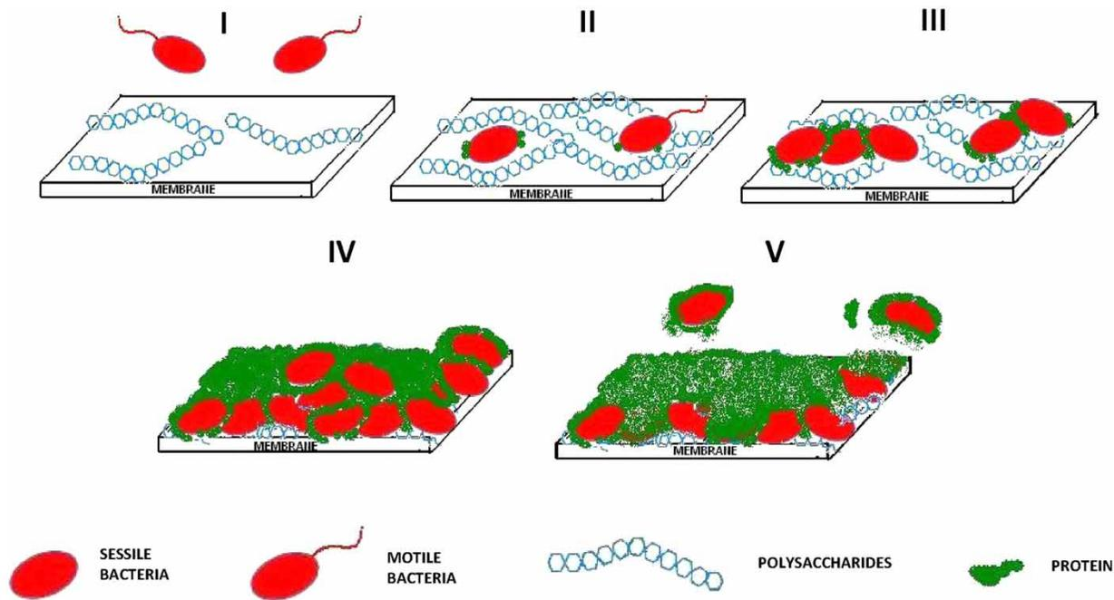
Figure 8 | A proposed mechanism for fouling biofilm.
