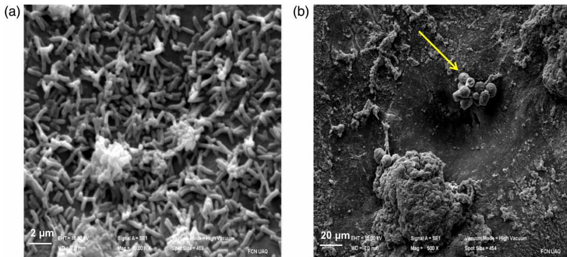
**Figure 6** | SEM micrographs at day 15. (a) Superficial fouling biofilm (monolayer); (b) bacterial clusters (granular-kind) and protozoa (arrow) growing on the biofilm bacterial monolayer.
