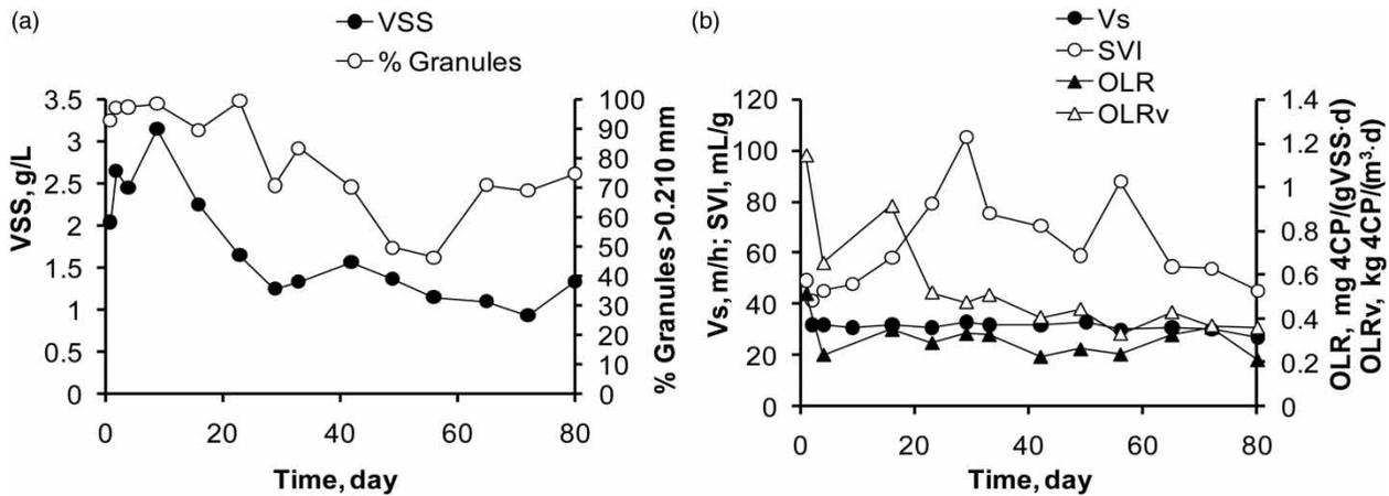
**Figure 2** | (a) Variation in biomass concentration and granulation percentage and (b) sludge volumetric index (SVI), settling velocity ( $V_s$ ), volumetric organic loading rate (OLRv) and organic loading rate (OLR) during the operation of the MSBR.
