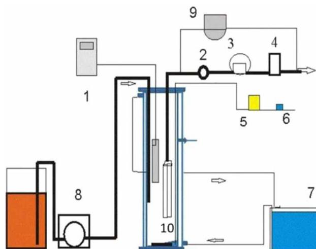
**Figure 1** | Schematic set-up of the membrane sequencing batch reactor. (1) Oxygen meter; (2) pressure gauge; (3) pump; (4) flow meter; (5) mass flow controller; (6) air-supplying valve; (7) water temperature device; (8) feeding pump; (9) backwashing pump; (10) membrane.
