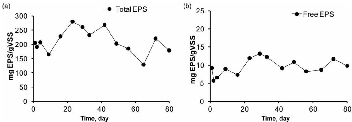
**Figure 3** | Total (a) and free (b) EPS obtained during the membrane operation.
