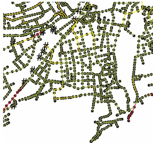
**Figure 6** | Vulnerability assessment for sewer collapse.
