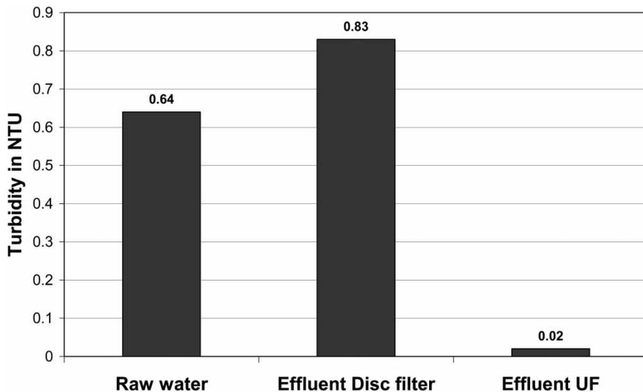
**Figure 3** | Turbidity in NTU for stored drinking water as raw water, after treatment by disc filter and after ultrafiltration.
