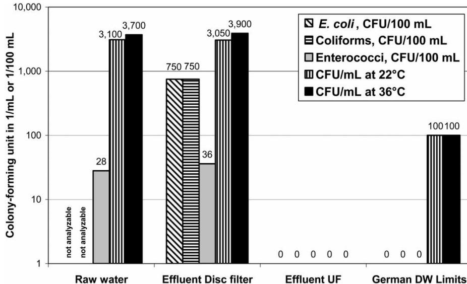
**Figure 4** | *E. coli*, coliforms, enterococci and total colony-forming units at 22 and 36 °C in log-scale for raw water stocked with wastewater, after treatment by disc filter and after ultrafiltration compared to German drinking water limits.
