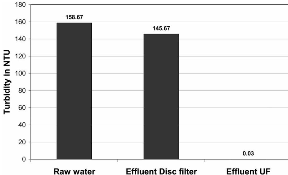
Figure 5 | Turbidity in NTU for raw water stocked with powdered activated carbon, after treatment by disc filter and after ultrafiltration.
