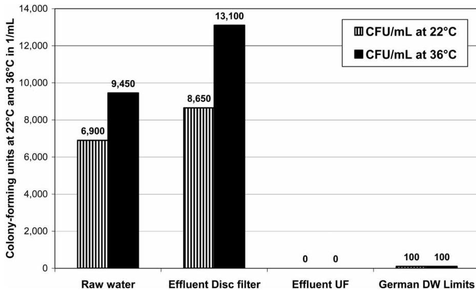
**Figure 2** | Total colony-forming units at 22 and 36 °C for stored drinking water as raw water, after treatment by disc filter and after ultrafiltration compared with German drinking water limits.
