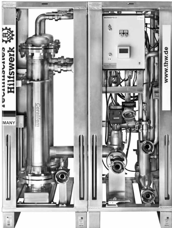
**Figure 1** | Picture of the UF module.
