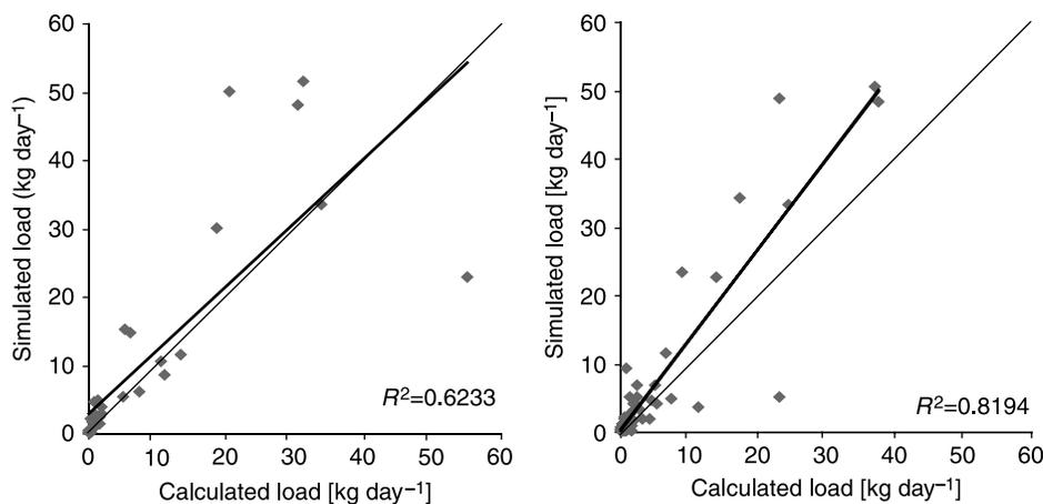
**Figure 3** | The simulated and calculated daily loads in the Loimijoki river basin. (a) Calibration period 1995–1999, (b) validation period 2000–2004.
