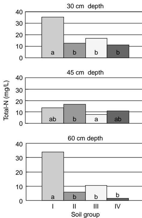
Figure 5 | Statistical comparisons ( $\alpha = 0.05$ ) of mean total-N concentrations eluted from each soil group at 30, 45 and 60 cm soil thickness treatments.
