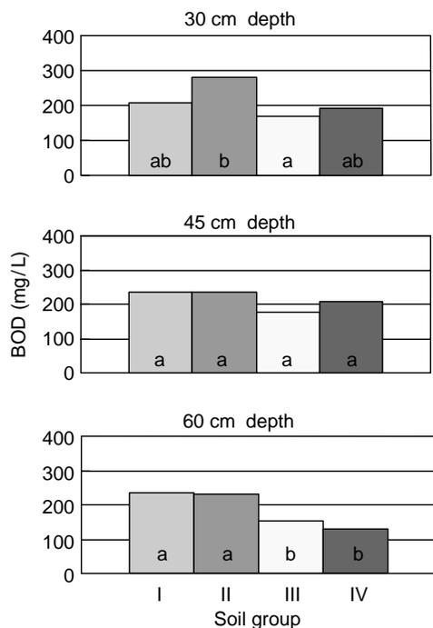
Figure 2 | Statistical comparisons ( $\alpha = 0.05$ ) of mean BOD concentrations eluted from each soil group at 30, 45 and 60 cm soil thickness treatments.
