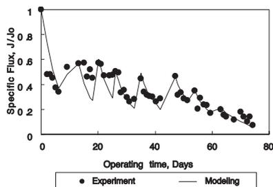
**Figure 3** Data fitting for finding the value of specific resistance and  $k_m$
