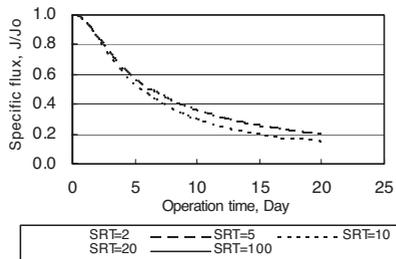
**Figure 5** Specific flux variation with operation time for different SRT
