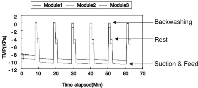
**Figure 2** Variation of trans-membrane pressure during operation
