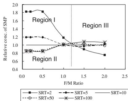
**Figure 6** SMP variation in the bioreactor with F/M ratio for different SRT
