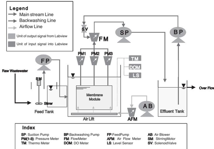
**Figure 1** Schematic diagram of the bench-scale SMBR system
