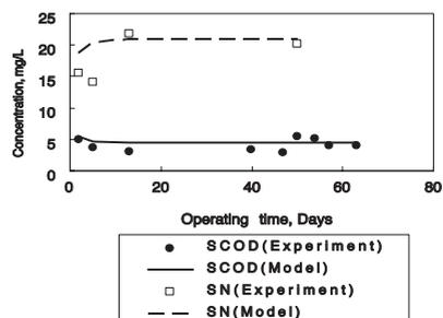
**Figure 4** Comparing simulation results with the soluble COD and nitrogen data from bench scale MBR
