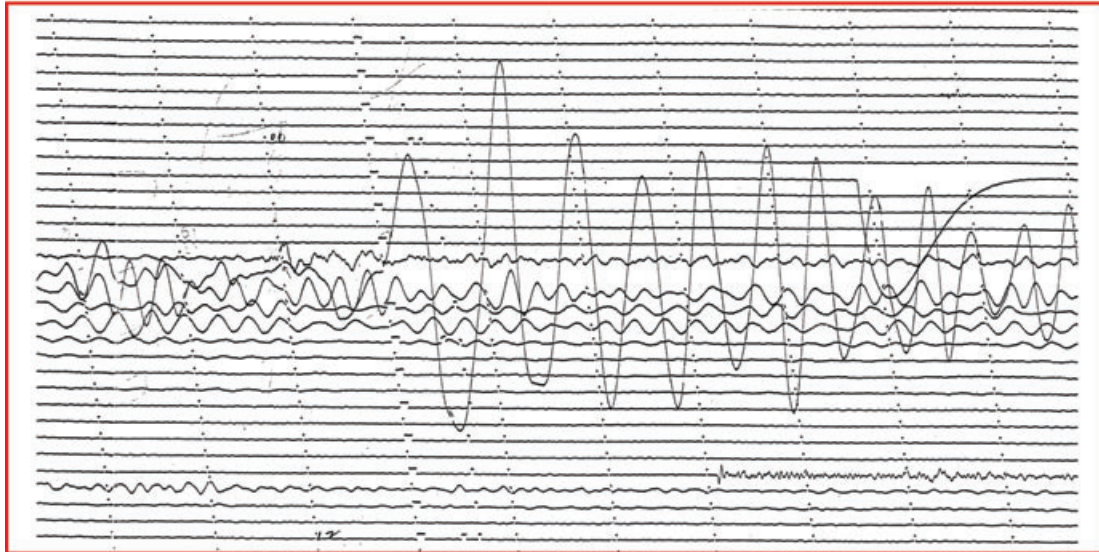
Figure 4. Example of record used in the PDFM inversion. This is the Rayleigh wave R_1 recorded on the vertical Benioff 1-90 instrument at Pasadena.
