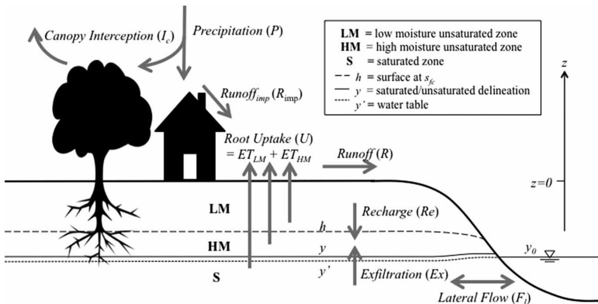
Figure 1 | Schematic of soil column and model framework (adapted from Laio et al. 2009).
