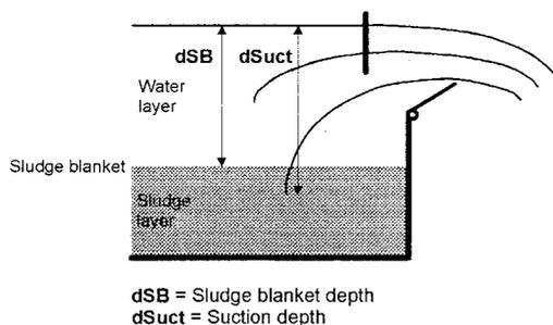
Figure 2 Parameter definition for modelling effluent SS
