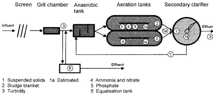
Figure 6 Description of the Aalborg East alternating WWTP
