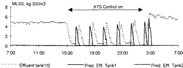
Figure 7 Measured and modelled MLSS out of aeration tanks
