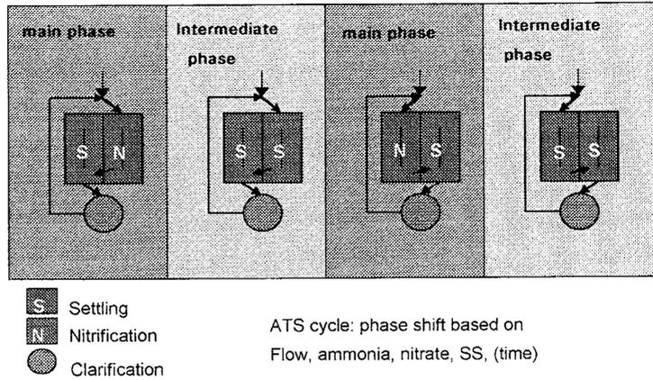
**Figure 1** Dynamic phase length control schemes for STAR control
