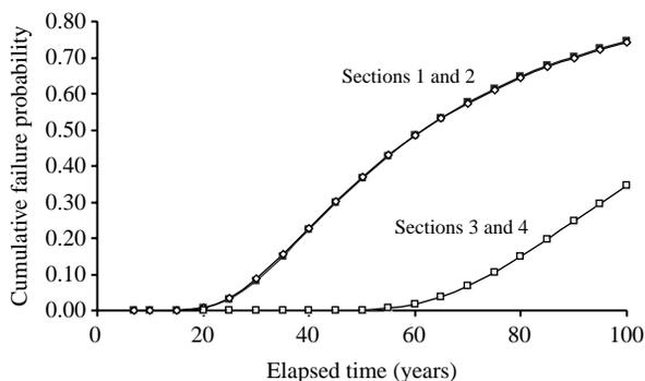
**Figure 5** | Cumulative failure probability for an individual 12 m long MSCL pipe.
