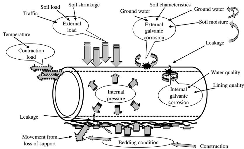
**Figure 2** | Galvanic corrosion process and failure causes in iron-based water pipe (based on O'Day 1988).
