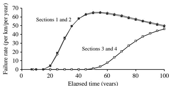
Figure 6 | Statistically expected failure rate for MSCL pipeline.
