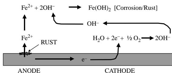
Figure 1 | Galvanic corrosion process in iron.
