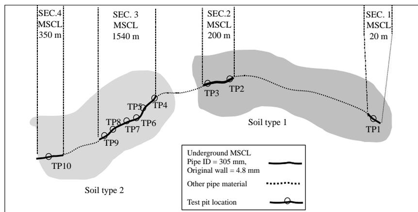
Figure 4 | Schematic layout of buried MSCL pipeline subject to external surface corrosion.
