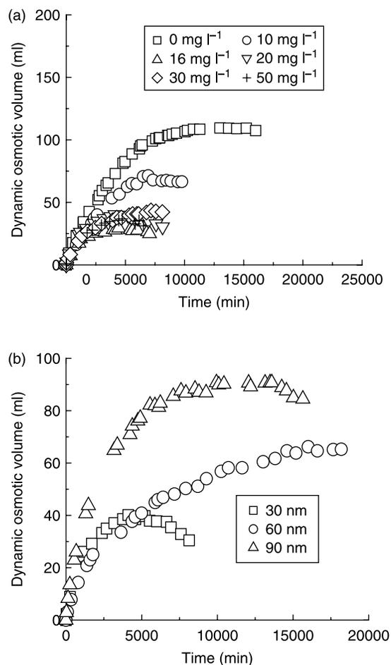
**Figure 7** | Influence of (a) concentration and (b) size of nano-colloids on dynamic osmotic volume (i.e. experimentally determined water volume flowing from permeate to feed sides) for ESNA1-LF membrane.
