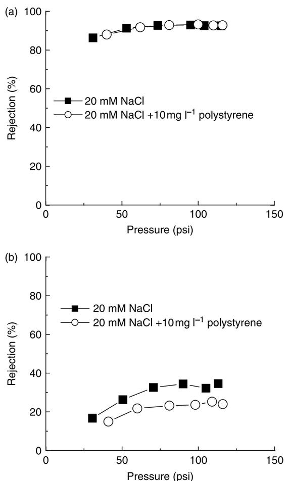
**Figure 6** | Ion rejection with respect to trans-membrane pressure in the presence of nano-colloids (30 nm, 10 mg l<sup>-1</sup>): (a) ESNA1-LF and (b) HL.
