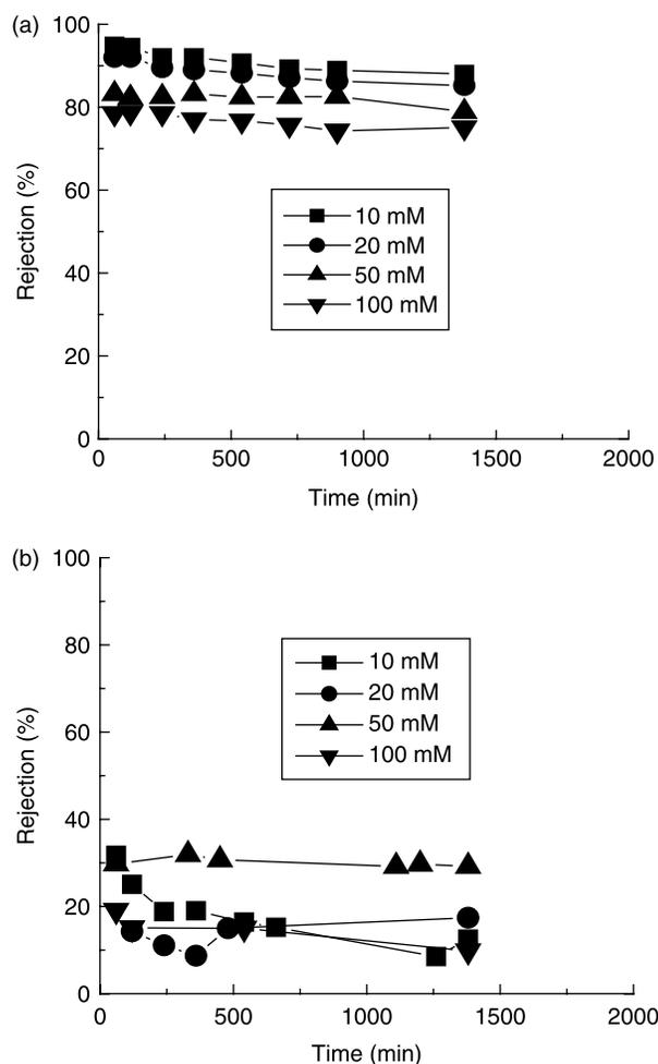
**Figure 4** | Influence of nano-colloids ( $30 \text{ nm}$ ,  $10 \text{ mg l}^{-1}$ ) on ion rejection at different feed water NaCl concentrations: (a) ESNA1-LF and (b) HL.
