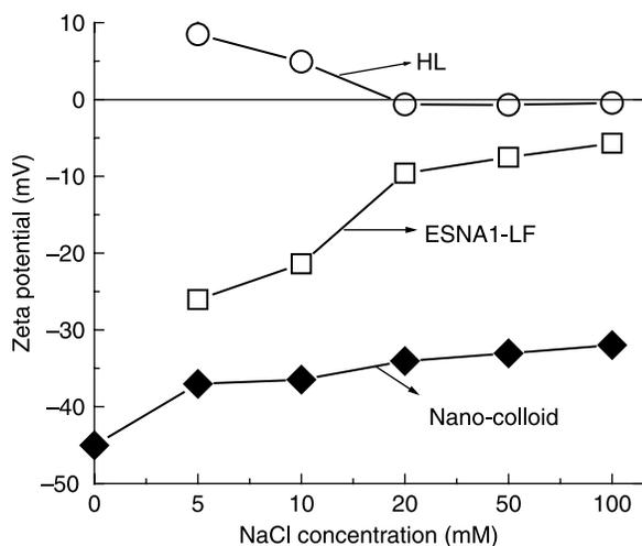
**Figure 2** | Zeta potentials of the NF membranes and nano-colloids as a function of NaCl concentration (pH 6.0).
