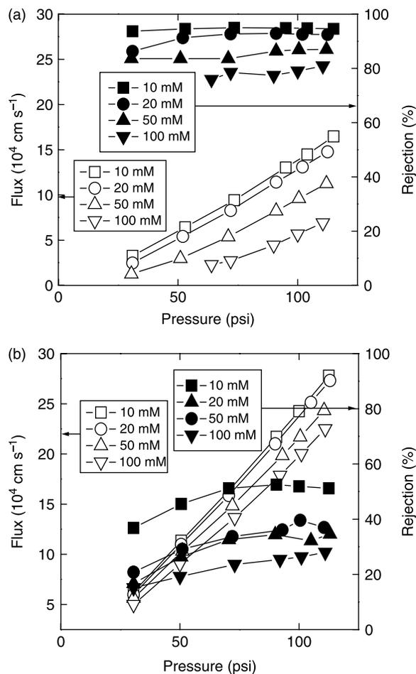
**Figure 5** | Ion rejection with respect to trans-membrane pressures at different feed water NaCl concentrations: (a) ESNA1-LF and (b) HL.
