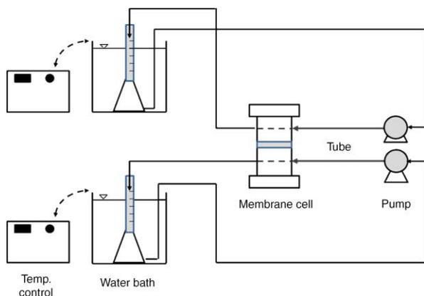
**Figure 1** | Schematic diagram of the osmometer system designed in this study.
