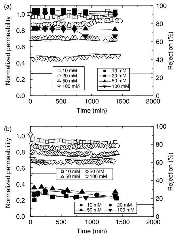
**Figure 3** | Normalized water permeability (open symbols) and ion rejection (closed symbols) at different feed water NaCl concentrations: (a) ESNA1-LF and (b) HL. Normalization was carried out based on pure water permeability.
