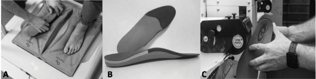
**Figure 2: Thermoforming the orthotic insoles (A); Orthotic insoles in ethinyl vinyl acetate, resin, and polyethylene (B); Further shaping the orthotic insoles (C)**
