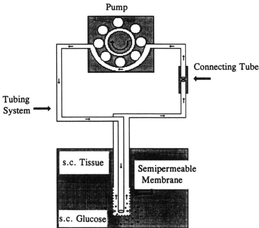
**Figure 1**—Recirculation method. Subcutaneous glucose diffuses into the recirculator following a concentration gradient. PBS is recirculated by means of a peristaltic pump in the tubing system; arrows indicate the perfusion direction. The connecting tube allows the recirculator to empty and refill.
