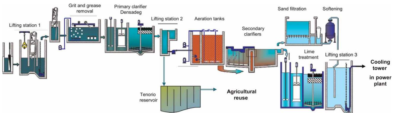
Figure 1 | Flow diagram of the treatment process.
