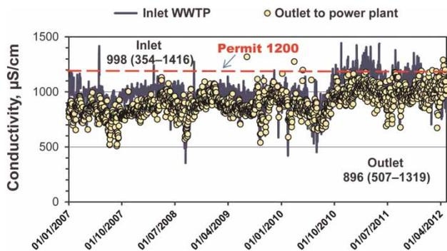
**Figure 4** | Evolution of the conductivity in secondary effluent for a 6-year period (2007–2012).
