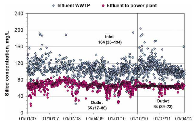
**Figure 5** | Evolution of the silica in secondary effluent for a 6-year period (2007–2012).
