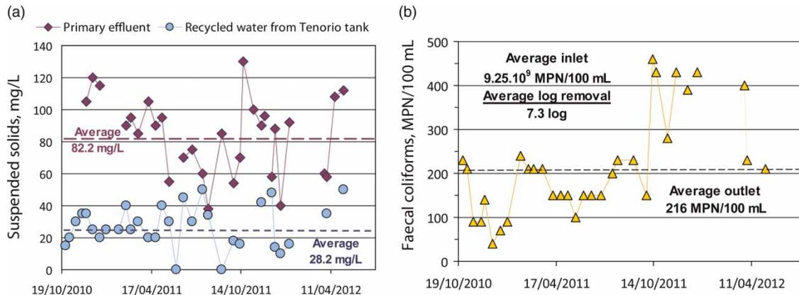
**Figure 3** | Evolution suspended solids (a) and faecal coliforms (b) in the outlet of the Tenorio Reservoir before the use for agricultural irrigation.
