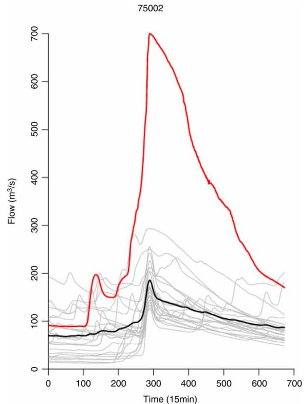
**Figure 9** | POT hydrograph plot for the period 2003–2009 for Camerton station at Workington (75002), showing mean hydrograph in black and the November 2009 event as a dotted line. The units on the x-axis represent number of 15 min time steps.
