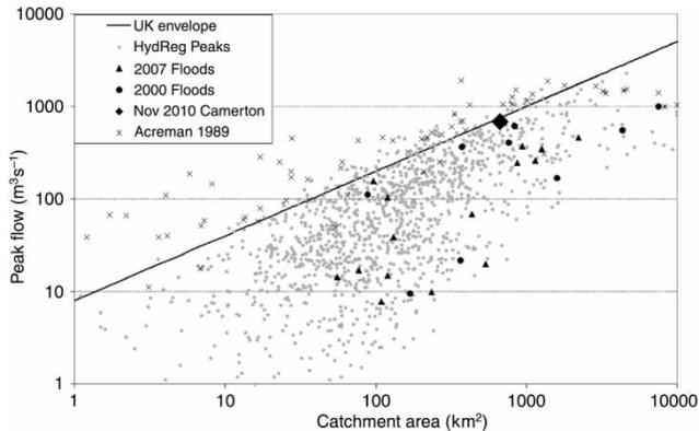
**Figure 12** | Maximum recorded flow in relation to catchment area for 1300 UK gauging stations contained within the UK hydrometric register (Marsh & Hannaford 2008) and 68 historical floods at un-gauged UK locations (Acreman 1989); plus Herschy (2002) UK flood envelope curve.
