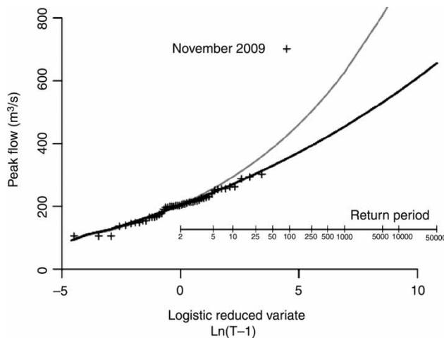
**Figure 4** | Flood frequency curves (pooled method) for the River Derwent at Camerton (75002) prior to the November 2009 event (black) and including the event (grey).
