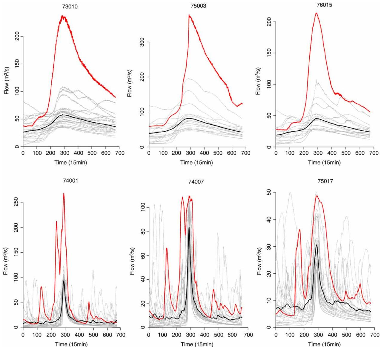
**Figure 8** | POT hydrographs for period 2003–2009 for lake-influenced catchments (above) and non-lake-influenced catchments (below), with the mean flood hydrograph denoted by the dark black line and the November 2009 event as a dotted line. The units on the *x*-axis represent number of 15 min time steps.
