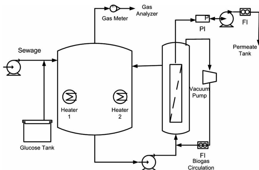
Figure 1 | Schematic of the pilot AnSMBR.
