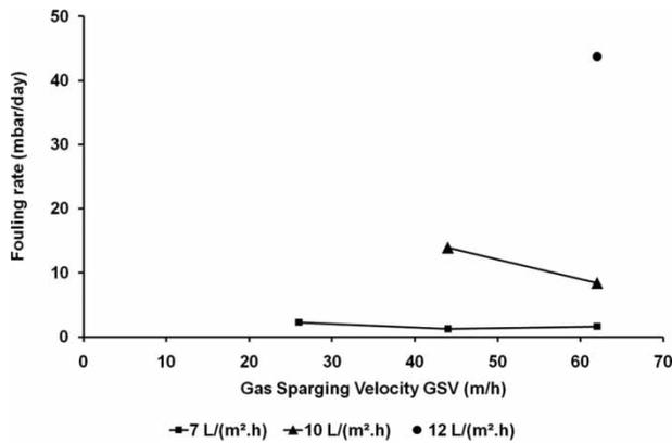
Figure 3 | Effect of the gas sparging velocity on the fouling rate. TSS: 14 g/L.
