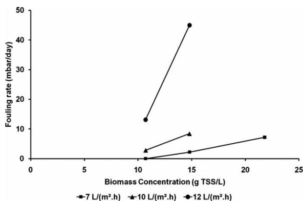
Figure 4 | Effect of the biomass concentration on the fouling rate. GSV: 62 m/h.
