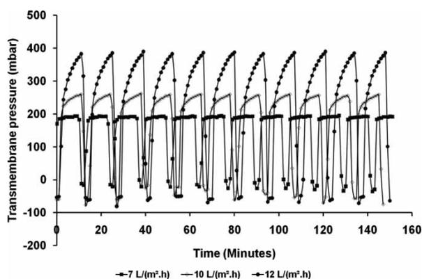
Figure 2 | TMP profiles at different fluxes in the short term. GSV:  $62 \text{ m/h}$ . TSS:  $14.9 \pm 0.9 \text{ g/L}$ .
