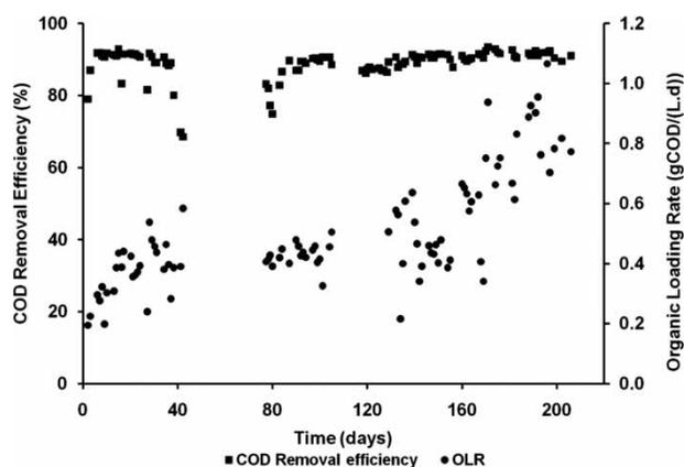
Figure 5 | COD removal efficiency and organic loading rate in time.
