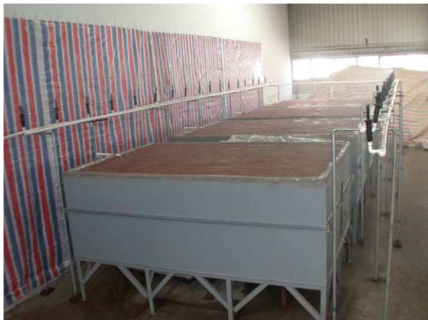
Figure 1 | View of different porous pavement test cells.
