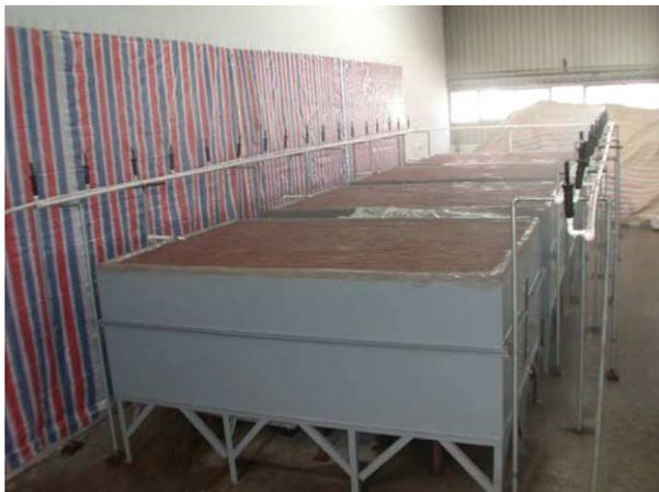
Figure 1 | View of different porous pavement test cells.
