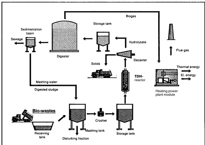
**Figure 1** Treatment of organic wastes by Thermal Hydrolysis (TDH) and subsequent biogas production by anaerobic digestion
