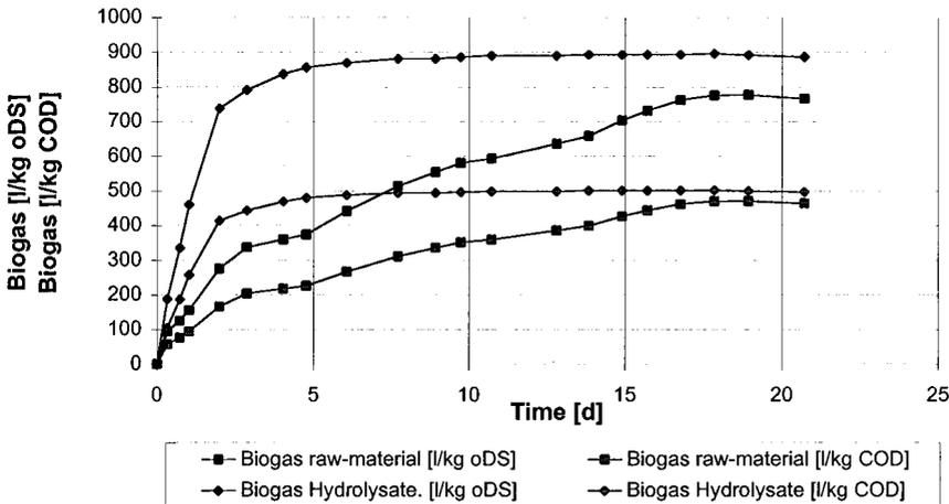
**Figure 3** Biogas production of the TDH - hydrolysate compared to the non hydrolyzed raw-material in the laboratory batch scale
